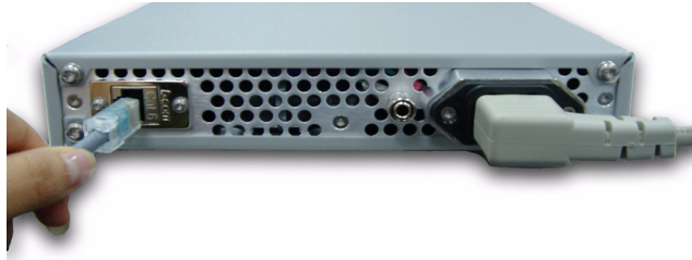
Figure 1-12 Connecting the LAN cable.
